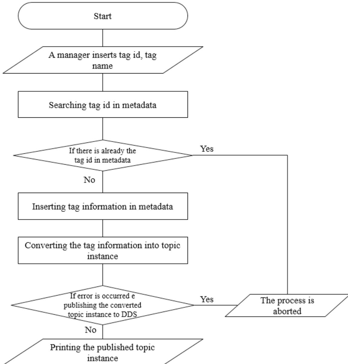
Figure 5. Flow chart for run-time (case2).
