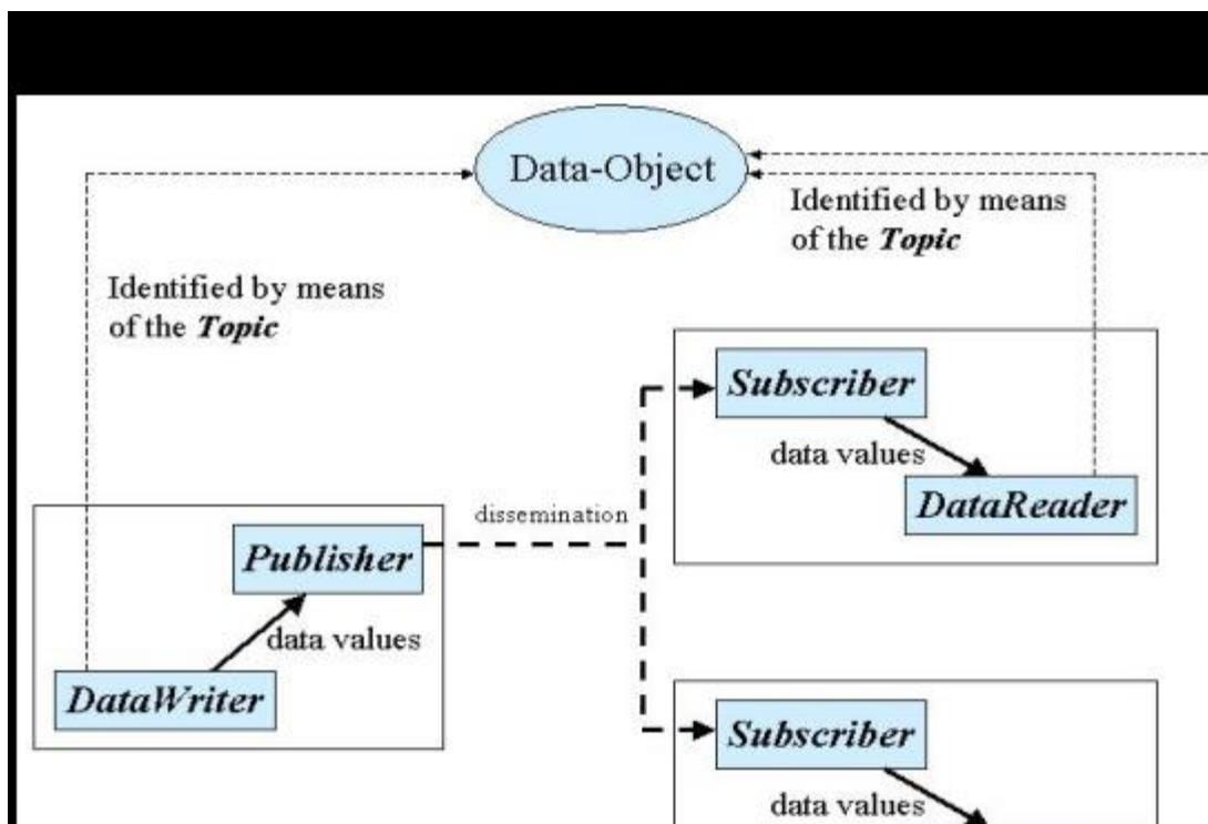
Figure 1. Basic structure of DDS standard.
