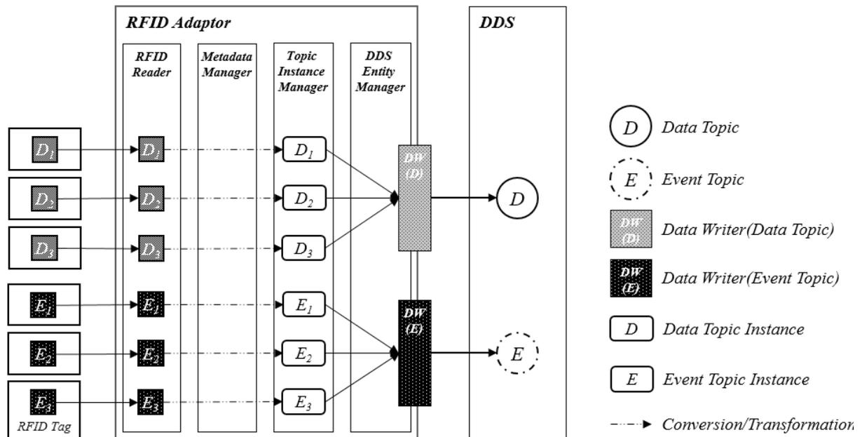
Figure 4. Components of RFID adaptor.
