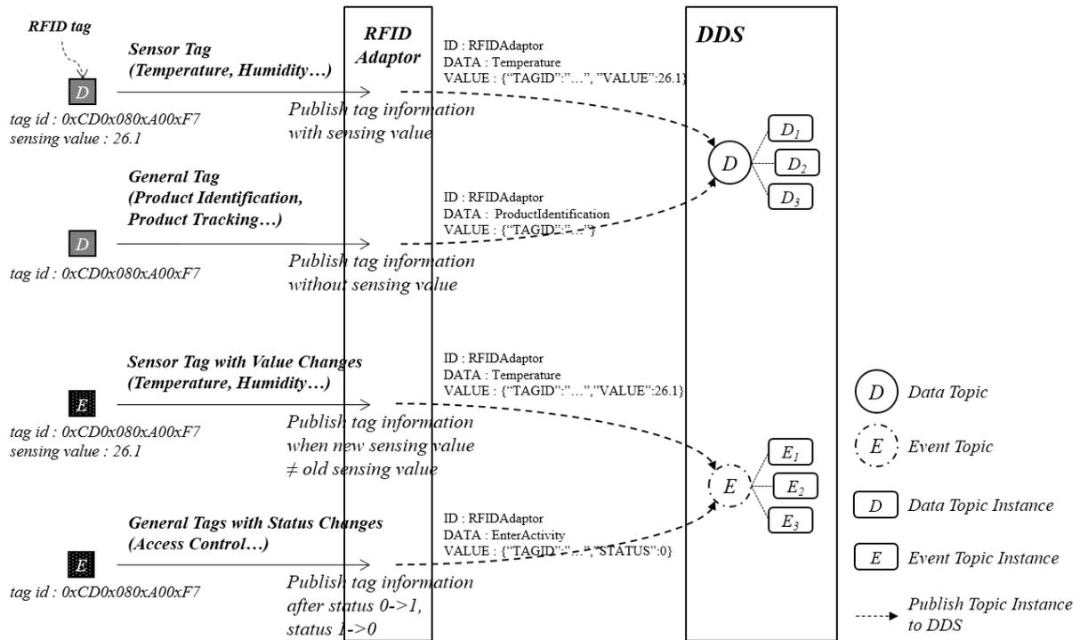
Figure 2. Example of data and events in RFID adaptor.
