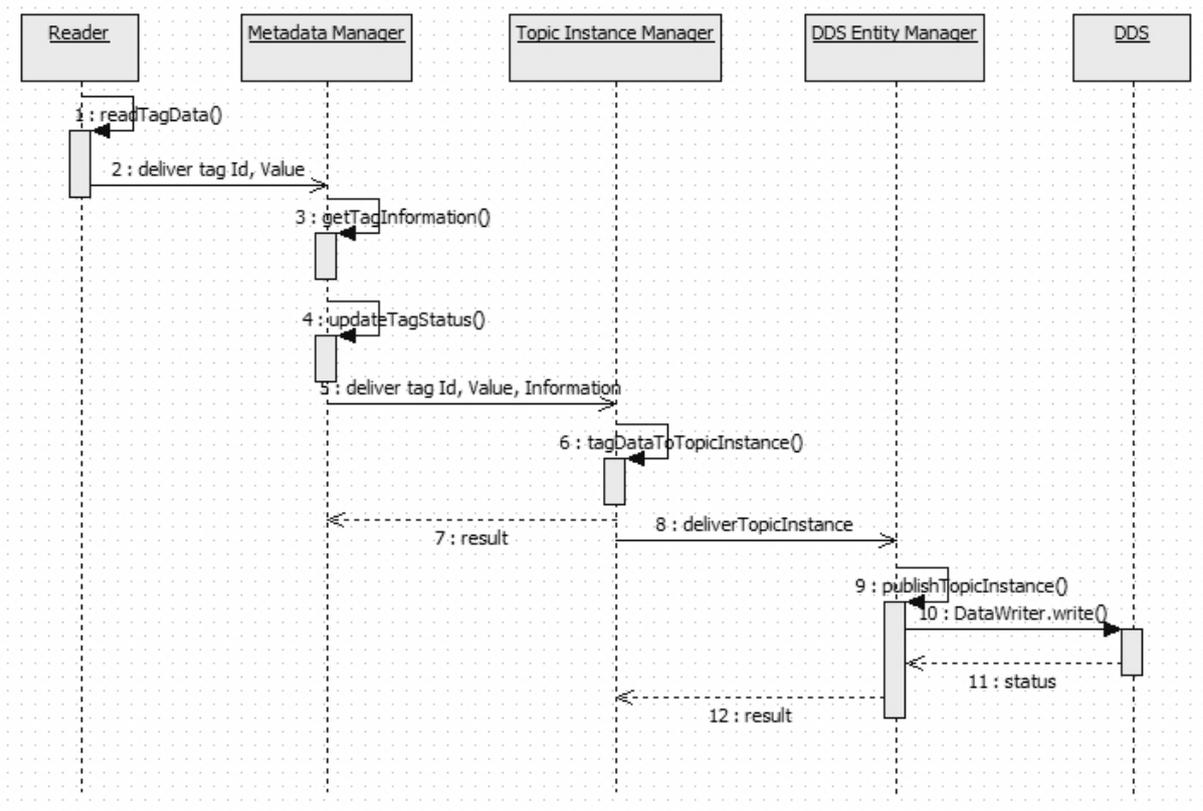
Figure 6. Sequence diagram for run-time (case 4).
